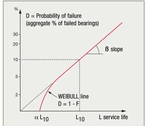
■ To take into account these facts in the reliability calculations for short operating periods, SNR ROULEMENTS uses the previous formula corrected by a factor  $\alpha = 0,05$
