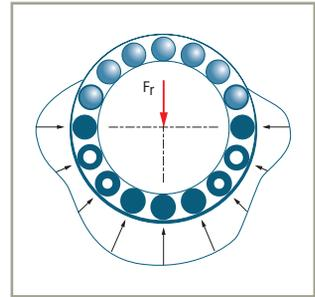
It is important for the bearing seats to be machined with a compatible level of precision. Seat shape defects (ovality, cylindricity defect, etc.) create local stresses that significantly reduce the service life of the bearings. Tables on page 108 give certain tolerance specifications for bearing contact surfaces and seats.
