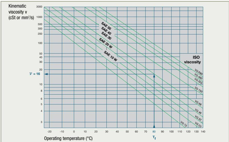
As the oil is defined by its nominal viscosity (in centistokes) at a nominal temperature of  $40^{\circ}\text{C}$  ( $104^{\circ}\text{F}$ ), its viscosity at the operating temperature is calculated from this.
