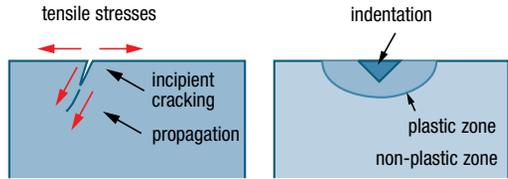
Considering the diversity of the contaminating particles found in the oil of a mechanical component and its evolution when new and after running in, and also considering the nature of the rolling elements (rollers or balls), which are affected to a greater or lesser extent by the phenomenon of slipping, the failure is often a combination of the SSIS and DSIS types.
