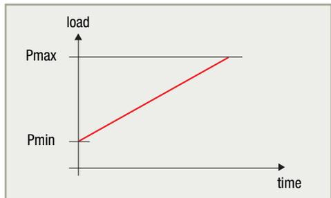
■ If the speed of rotation and the load are variable, the service life is calculated for each level of use, then the duration is weighted for the cycle as a whole.
