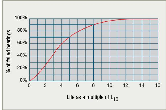
The reference for bearing life is the  $L_{10}$  duration which is given for a 90% reliability, or conversely, a 10% probability of failure. It is possible to calculate a service life for a different level of reliability using the factor  $a_1$ , or to find the reliability  $F$  for a chosen operating time.
